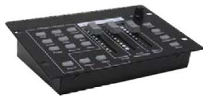
3-Channel DMX Controller 5ft 120V AC power cord plus adapter Nine color presets DMX-RGB-3
