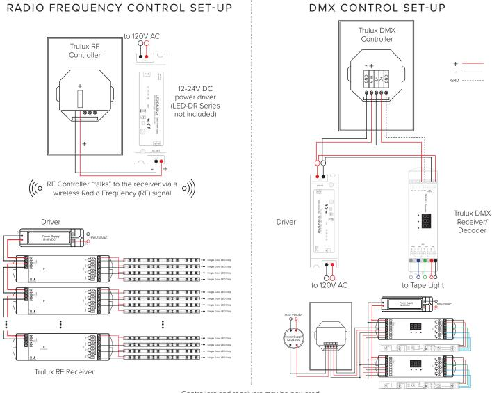
Controllers and receivers may be powered by the same driver on the secondary side
