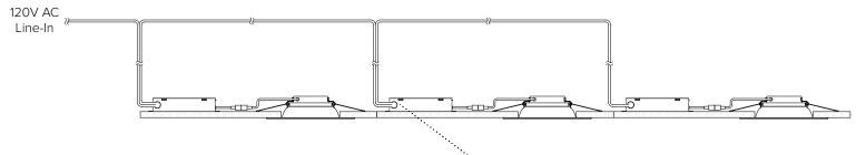
Each fixture includes a remote driver housed in an attached junction box with two knockouts (each driver is rated for use with the fixture it was included with)
